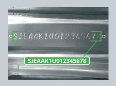
A highly configurable quality control inspection system – VINi - from Industrial Vision Systems lets you automate repetitive critical inspection of your VIN and serial number scribes with high accuracy. VINi uses artificial intelligence to provide mission critical character recognition and quality inspection criteria across the entire production marking cycle.
